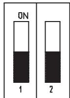
**DIP 1 OFF****DIP 2 OFF****2. SETTING THE OPERATING LOGIC WITH A SENSOR DEVICE**
